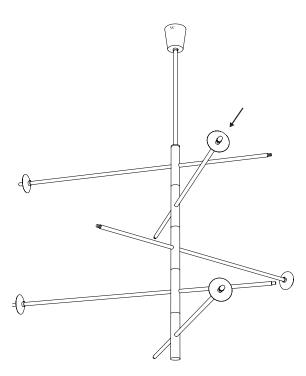
Screw brass spheres from bottom to top.
