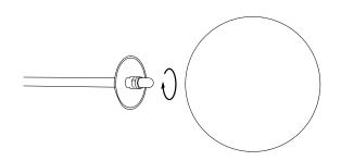
Screw the glass globe up to the resistor. Beware! Do not tighten stronger than natural resistance.
