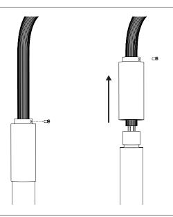
To change the neon tube, unscrew the retainer screw and slide the brass cylinder.
