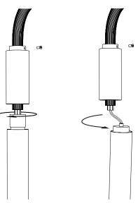
Unscrew the metal piece to release the connectic part.
