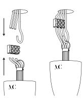
Connect the wires to the mains after setting up the hook.
