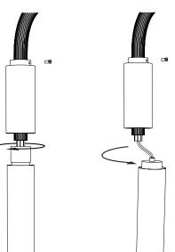
Unscrew the metal piece to release the connectic part.
