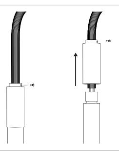
To change the neon tube, unscrew the retainer screw and slide the brass cylinder.
