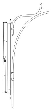
Fix the plate to the wall with dowels.
