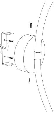
Fix the plate to the wall with dowels.
