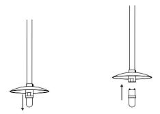
Insert the light source into the base
