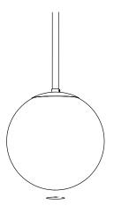
Screw the glass globe up to the resistor. Beware! Do not tighten stronger than natural resistance
