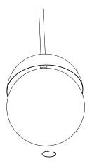
Screw the glass globe up to the resistor. Beware! Do not tighten stronger
