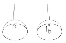
Insert the light source into the base.
