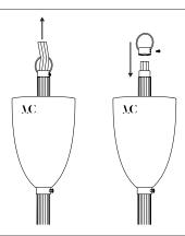
Unscrew the hook and insert the wires before screw it back.
