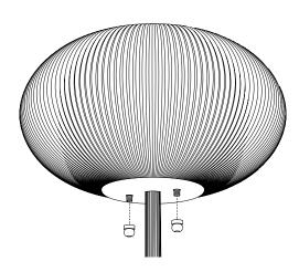
Unscrew the two brass pieces while holding the glass.
