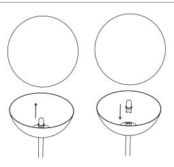
Insert the light source into the base.
