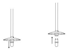
Insert the light source into the base.
