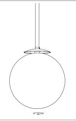
On the case of light bulb remplacement. Unscrew the glass globe.
