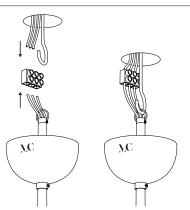
Connect the wires to the mains after setting up the hook.
