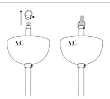
Unscrew the hook and insert the wires before screw it back.
