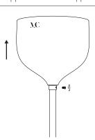
Pull up the thread guard after unscrewing the ring's screw.
