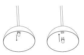
Insert the light source into the base.
