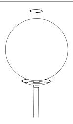
Screw the glass globe up to the resistor.
