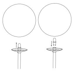
Insert the light source into the base.
