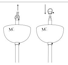
Unscrew the hook and insert the wires before screw it back.
