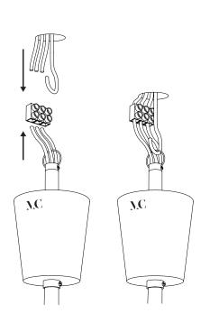
Connect the wires to the mains after setting up the hook.
