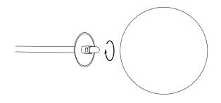
Screw the glass globe up to the resistor. Beware! Do not tighten stronger
