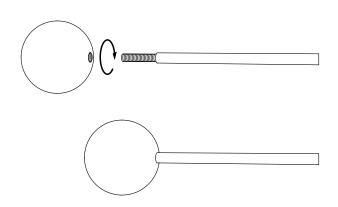
The brass spheres are screwed to threaded tubes.
