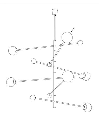
Screw glass spheres from bottom to top.
