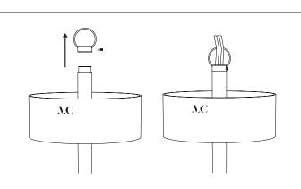
Connect the wires to the mains after setting up the hook.
