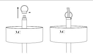
Unscrew the hook and insert the wires before screw it back.
