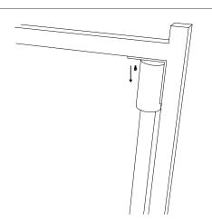
In case of neon tubes replacement, unscrew the screw.
