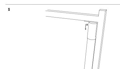
In case of neon tubes replacement, unscrew the screw.
