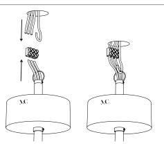
Connect the wires to the mains after setting up the hook.
