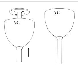
Pull up the thread guard by unscrewing the ring's screw and screw it back.
