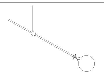
Screw the glass globe until the first sign of resistance. Do not tighten stronger than natural resistance.
