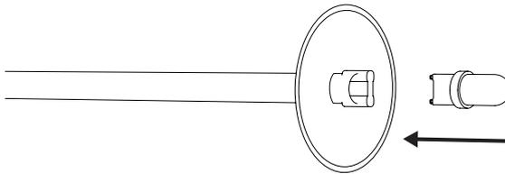
Insert the light source into the base.
