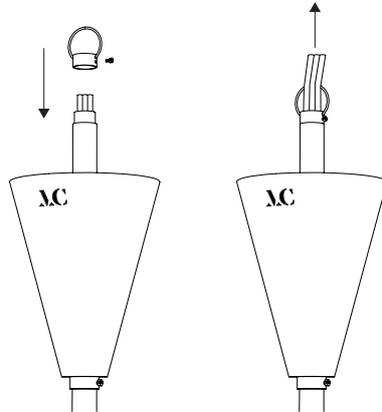
Unscrew the hook and insert the wires before screw it back.
