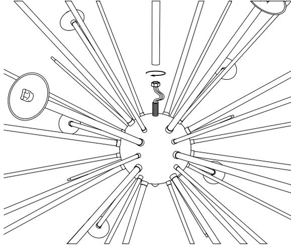
After removing all the walls of the transport box, unscrew the transport screw.
