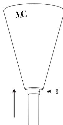
Pull up the thread guard after unscrewing the ring's screw.
