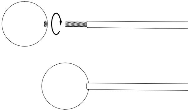
The brass spheres need to be screwed to threaded tubes.
