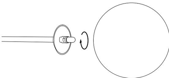
Screw the glass globe up to the resistor.
