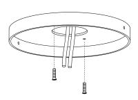
Fix the plate to the ceiling with dowels.
