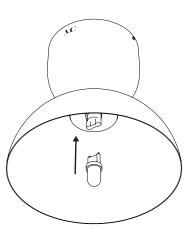
Insert the light source into the base.
