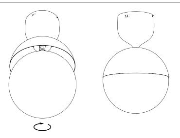
Screw the glass globe up to the resistor.
