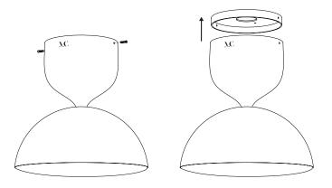
Free the plate by unscrewing the screws.
