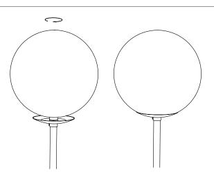
Screw the glass globe up to the resistor.
