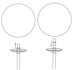
Insert the light source into the base.
