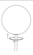
Unscrew the ring and pull up the cupola before screw it back.
