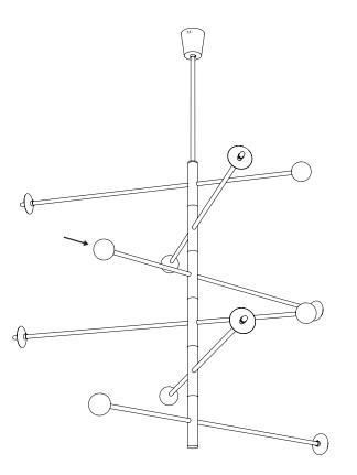
Screw brass spheres from bottom to top.
